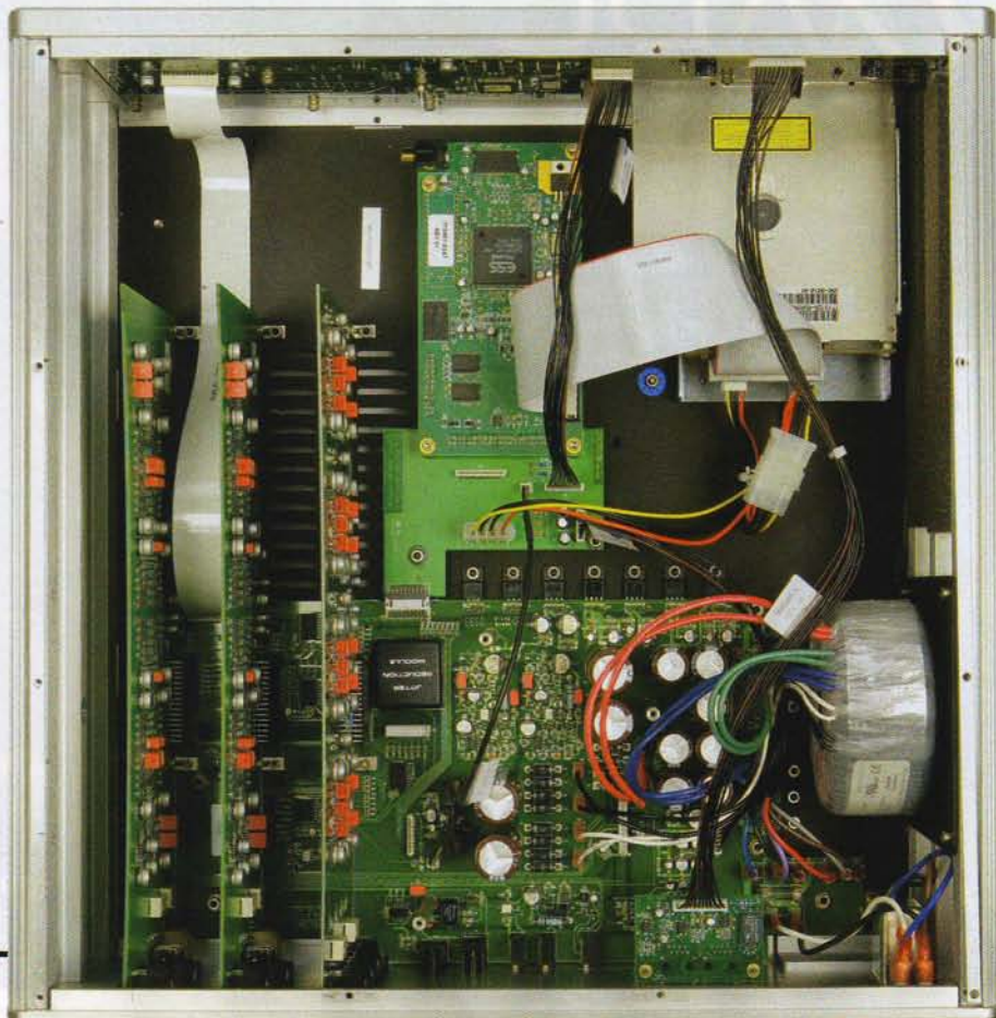
RIGHT: Multi-platform disc drive feeds two-channel DACs on the two leftmost vertical (analogue output) cards. The centremost board is equipped with DSD1793 DACs for the centre, surround and sub channels
